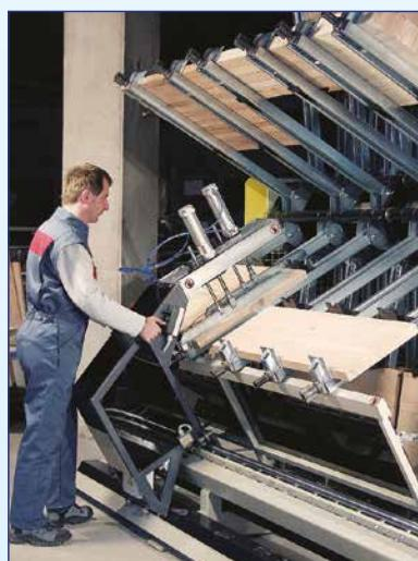
Pressure build-up is not activated until the signal is given by both hands at the same time.
