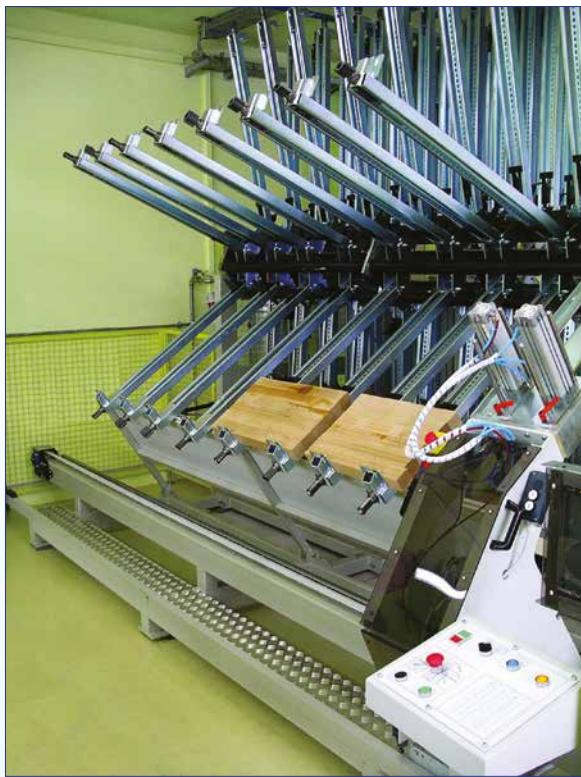
UK The clamp carrier Model SL – H is intended for edge gluing and lamination of wooden stock whose joints are dried naturally.
